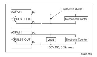
Figure 4.4.10 Pulse Output Connection
